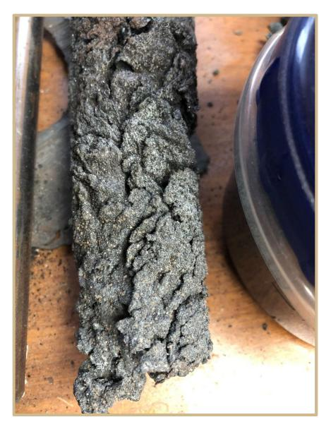
The result of a clogged ladle gate. Steel appears to have seeped down the channel where the sand is held, hardening prematurely and forming an interface with the sand. This led to the molten steel in the ladle unable to flow through the channel once the gate was opened. Image provided by Nucor Steel.
